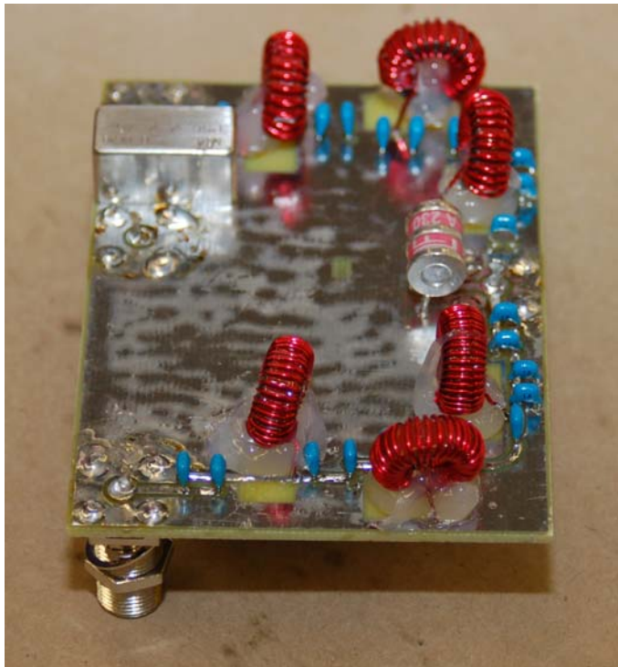
Figure 7 (second page): K3NA W3LPL bandpass filter-splitter.
