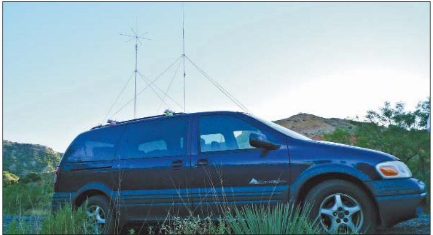
The mobile antenna farm for AD4EB's rover activities.
