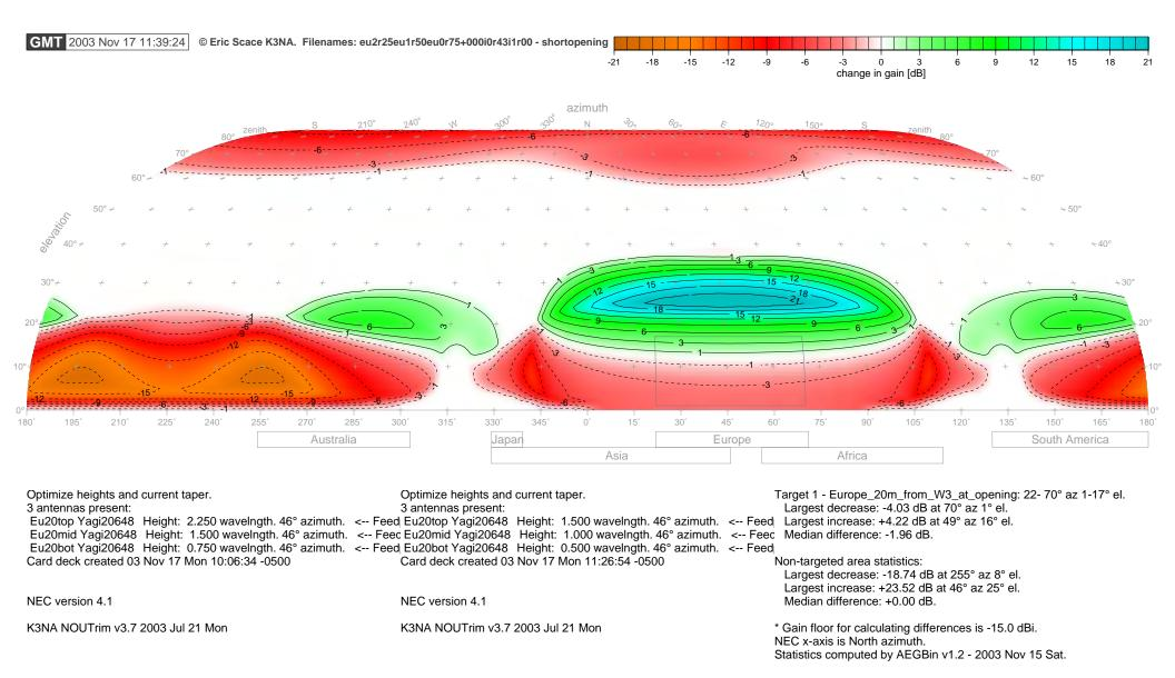
Figure 19 - Comparing current-tapered tall and short 3-Yagi stacks (Figures 18 and 14). The short stack is cleaner in zenith and rear but down -3 to -4 dB at low target elevations.
