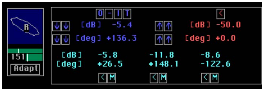
Figure 2 — The small window on the left is the Linrad polarization graph, which graphically displays phasing and amplitude balance. It is also used to set the time constant of the adaptive receive mode. The other window is a phasing window, an extension of the polarization graph which displays amplitude and phase information numerically. You can also use the controls in this window to manually adjust amplitude and phase.
