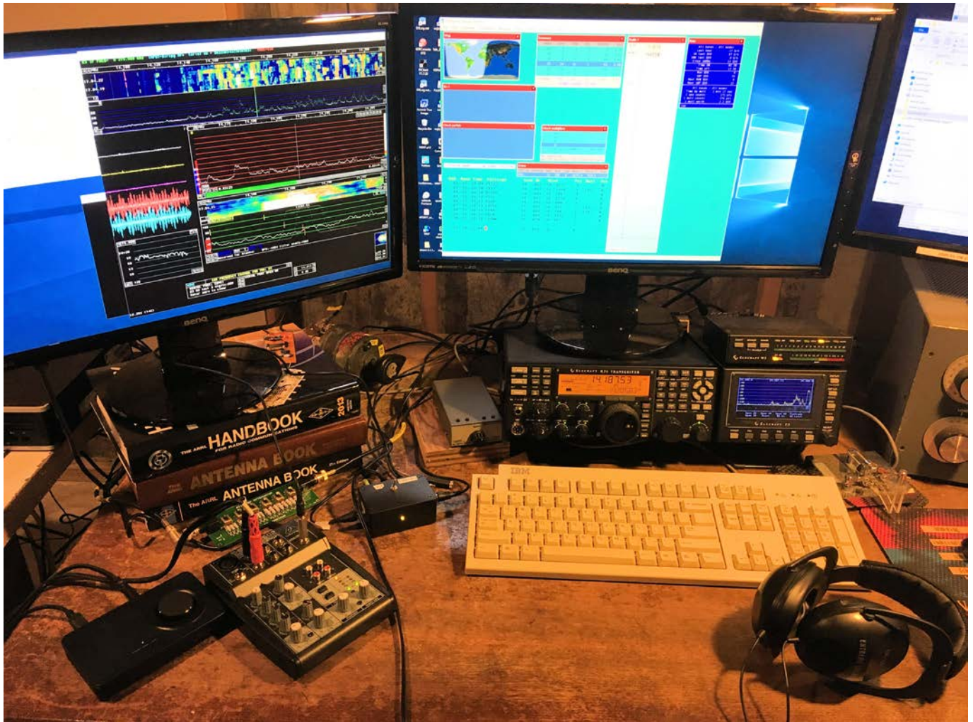
Figure 4 — My station running Linrad during the 2019 WPX SSB. The three boxes specific to using Linrad (left to right) are the Asus Xonar USB sound card, used as Linrad audio output; the Kenyx 502 mixer console, and the Linrad /K3 audio switchbox. Not shown is the very small Airspy HF+ SDR, plugged into the IF OUT port of the K3.
