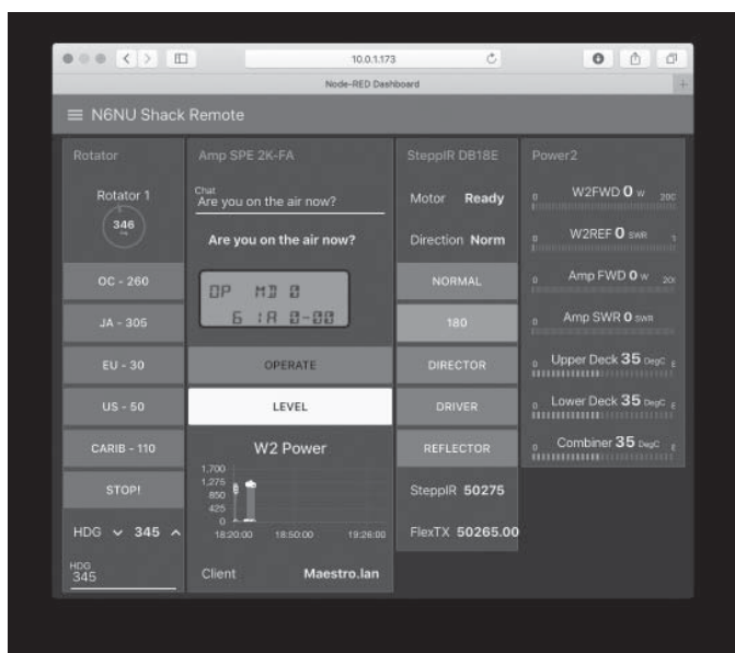
N6NU’s “Shack Remote” interface was developed in Node-RED for the Raspberry Pi. [Andreas Junge, N6NU, photo]
