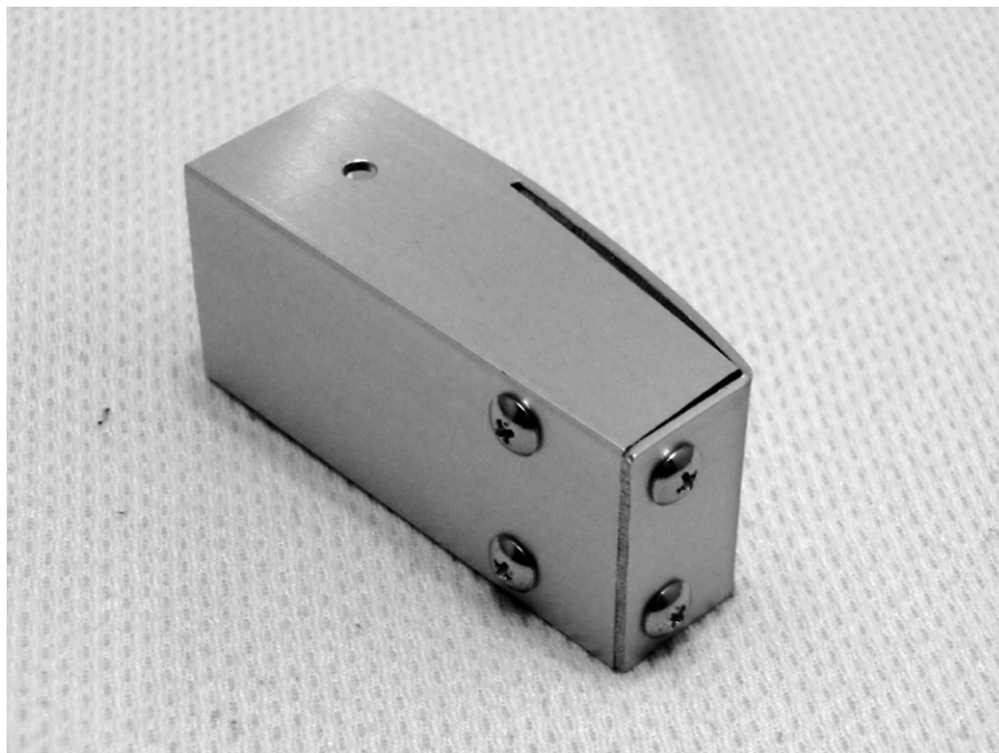
Figure 1 — Pieces of square aluminum stock frame the pedal opening. A "flap" is cut along one side of each, then trimmed to create a slight flare. The flap then is bent over to enclose the end.
