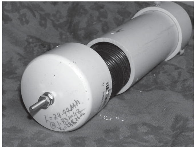
Figure 4 — Far end loading coil
