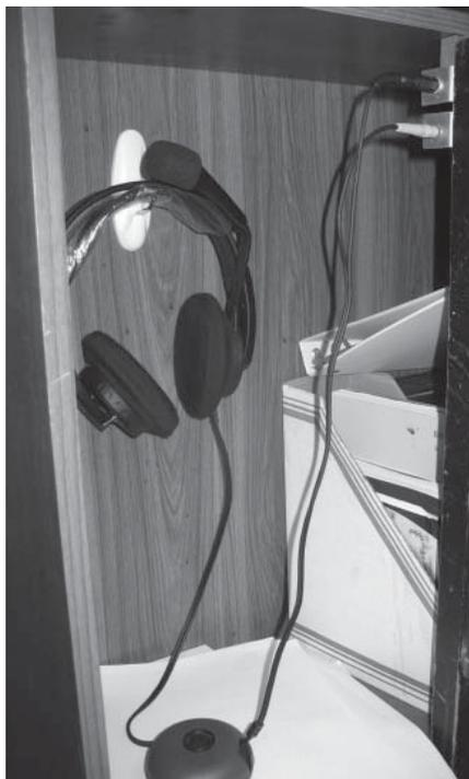
Figure 3 — Headphones hang at the left end of the desk return are plugged into jacks wired to radio via the patch bay. A cable roller stores excess cable.
