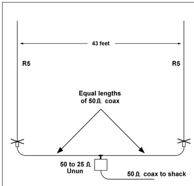
Figure 2 — System diagram for phased R5 verticals
