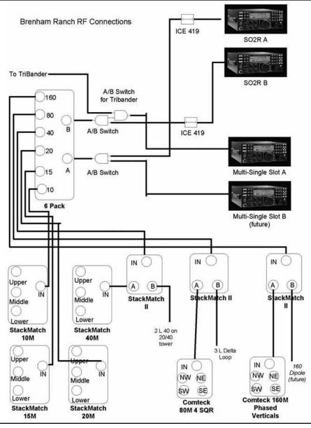
Figure 1 – Basic RF Path Layout
