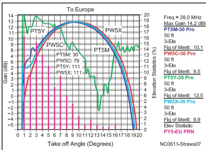
**Figure 7—HFTA response for Top Four stations toward Europe on 10 meters. The table of numbers shows the QSOs into Europe for each station. PT5Y would appear to have an advantage by about 2.5 dB on average over all the statistically relevant elevation angles.**
