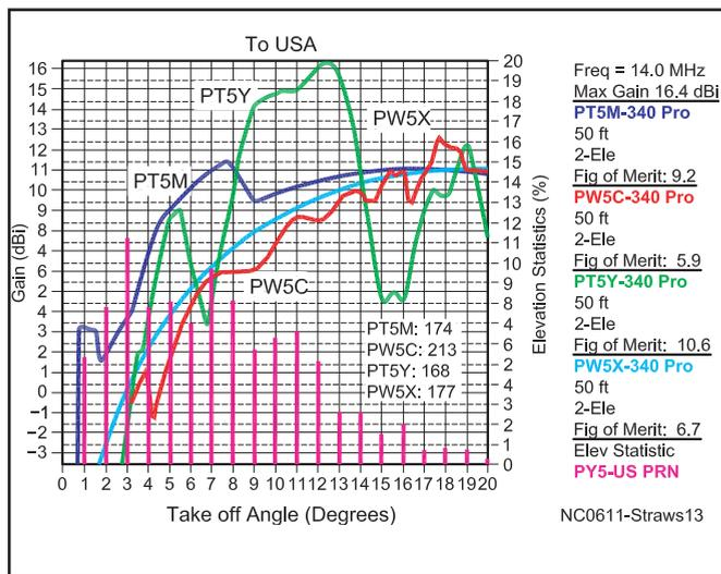
**Figure 13—Responses for Top Four stations toward the USA on 20 meters. Again, PT5M looks like it is nominally stronger into the USA on 20 at low elevation angles.**
