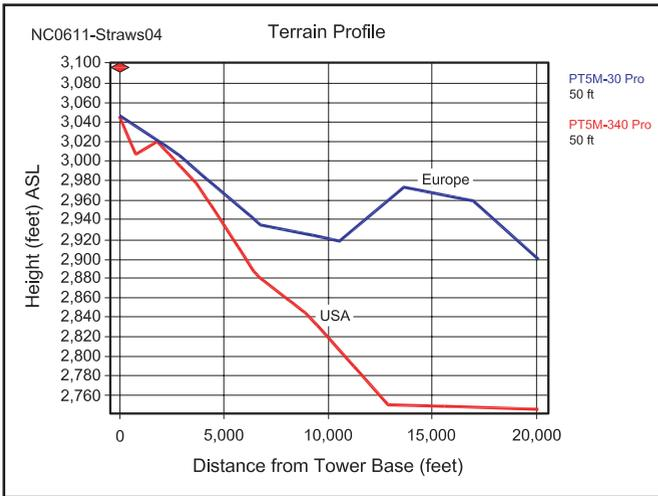
**Figure 4—Terrain profiles toward Europe and toward the USA from PT5M. The ground slopes down in both directions but the slopes are only about 1° due to differences in the x- and y-axes in this HFTA graph.**
