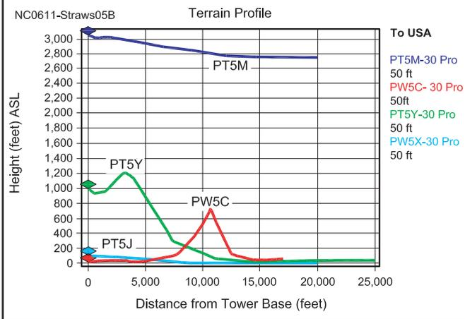
**Figure 5—At A, a “true-perspective” view of the terrain profiles toward Europe from the Top Four WRTC 2006 stations, using equal scaling on both x- and y-axes. The PT5Y terrain slopes down such that the equivalent height of the tri-band antenna on 15 meters was about 65 feet, compared to the actual physical height of 50 feet. At B, HFTA terrain profiles toward the USA.**
