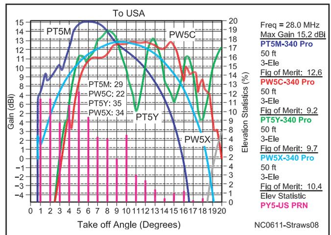
**Figure 8—Responses for Top Four stations toward the East Coast of the USA on 10 meters. PT5M appears to be top dog in this direction.**
