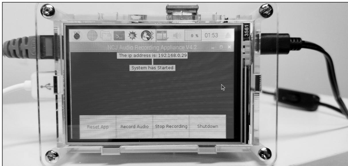
Figure 1 — The card with a 3.5-inch LCD touch screen with the Raspberry Pi on the back in a Plexiglass case.
