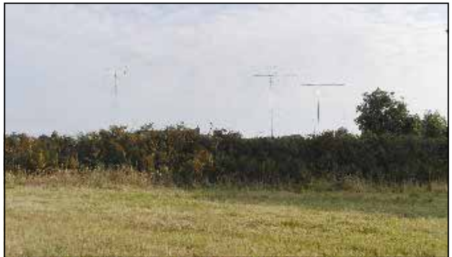
Antennas seen from the coastal path on the east of the island. 10/15-meter quad up 35 feet, TB33 tribander up 34 feet with a 6-meter Yagi above, and an 11-element 2-meter Yagi on a 29 foot pole to the right.
