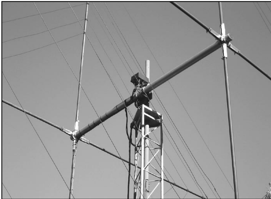
Figure 2 — A cardinal rule in quad design is to avoid tying all the elements together in the middle of the quad. Instead, use a remote antenna switch to swap the feed line among elements for each band.
