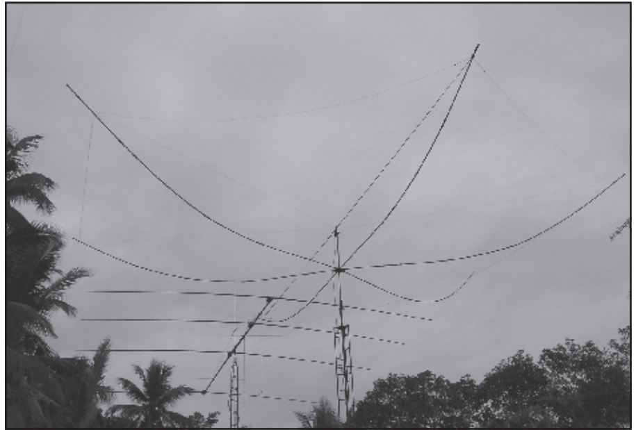
The 4S7AB antennas—a 4-element SteppIR in the back and a 40-meter homebrew Hex Beam in front.
