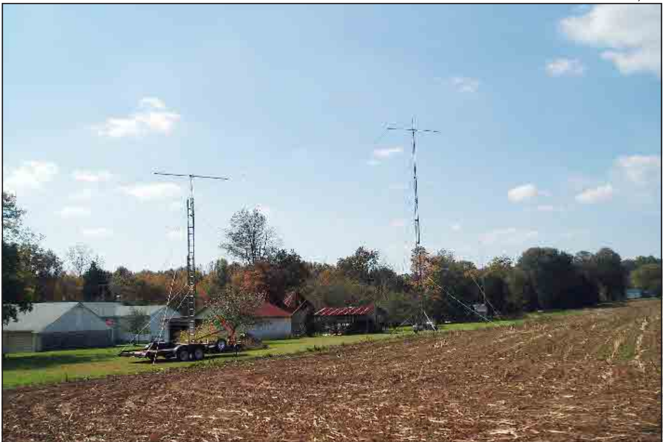
Three of the portable antennas we used: At the left is the ladder-mounted 15-meter beam. In the center is the club's trailer-mounted tower with the 4-element 20 meter beam. On the right is the 40-foot mast supporting the 40-meter delta loop. AI2C's farmhouse and outbuildings are in the background.
