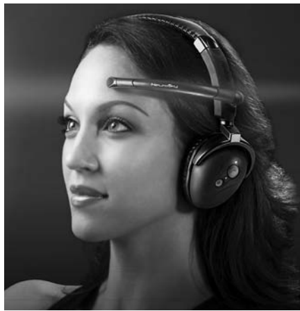
Figure 2 —The NeuroSky Mindset wireless headset, microphone and EEG: That's not a misplaced boom mic on her forehead. It's a sensor "listening" to her brain. NeuroSky, used with permission
