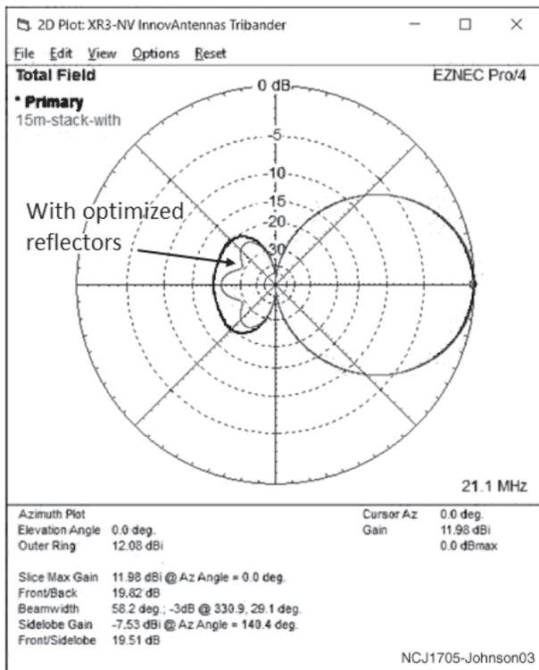
**Figure 3 — 15 meter stack results with sub-array of 2 x 15-meter optimized reflectors and without.**
