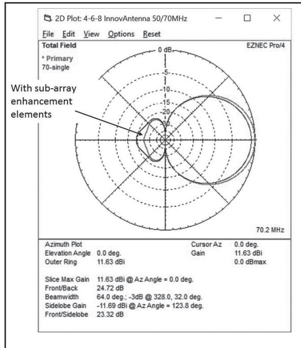
**Figure 5 — 70 MHz performance of a vertical stack of 8 element 50 MHz/70 MHz duo band yagis with and without sub array elements.**
