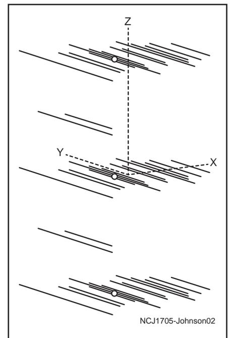
Figure 2 — Three stack of InnovAntennas/G0KSC XR3-NV triband Yagis with sub-reflector arrays.
