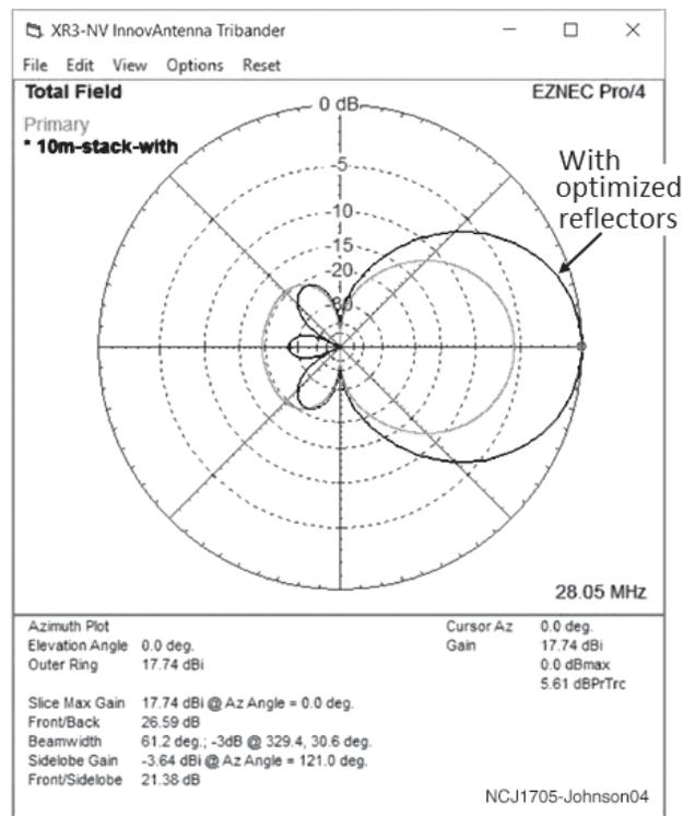
**Figure 4 — 10-meter stack enhancements with sub-array of 2 x optimized reflectors and without.**
