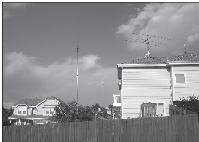
The 80/40-meter array in N0AH's backyard. That's a Cushcraft MB1020 beam on the roof of the house.
