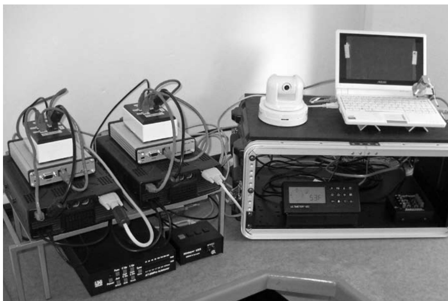
Figure 8 — New SO2R remote setup using Remoterig interface units at one end of new mini-barn shack desk
