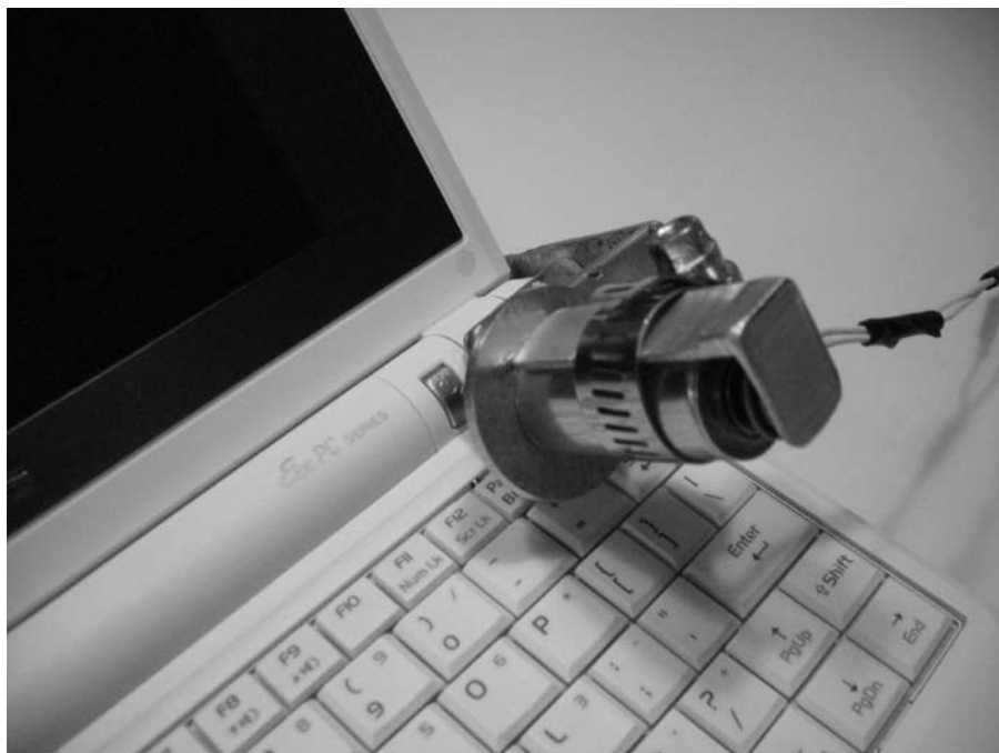
Figure 7 — The remotely controlled solenoid for powering on the computer
