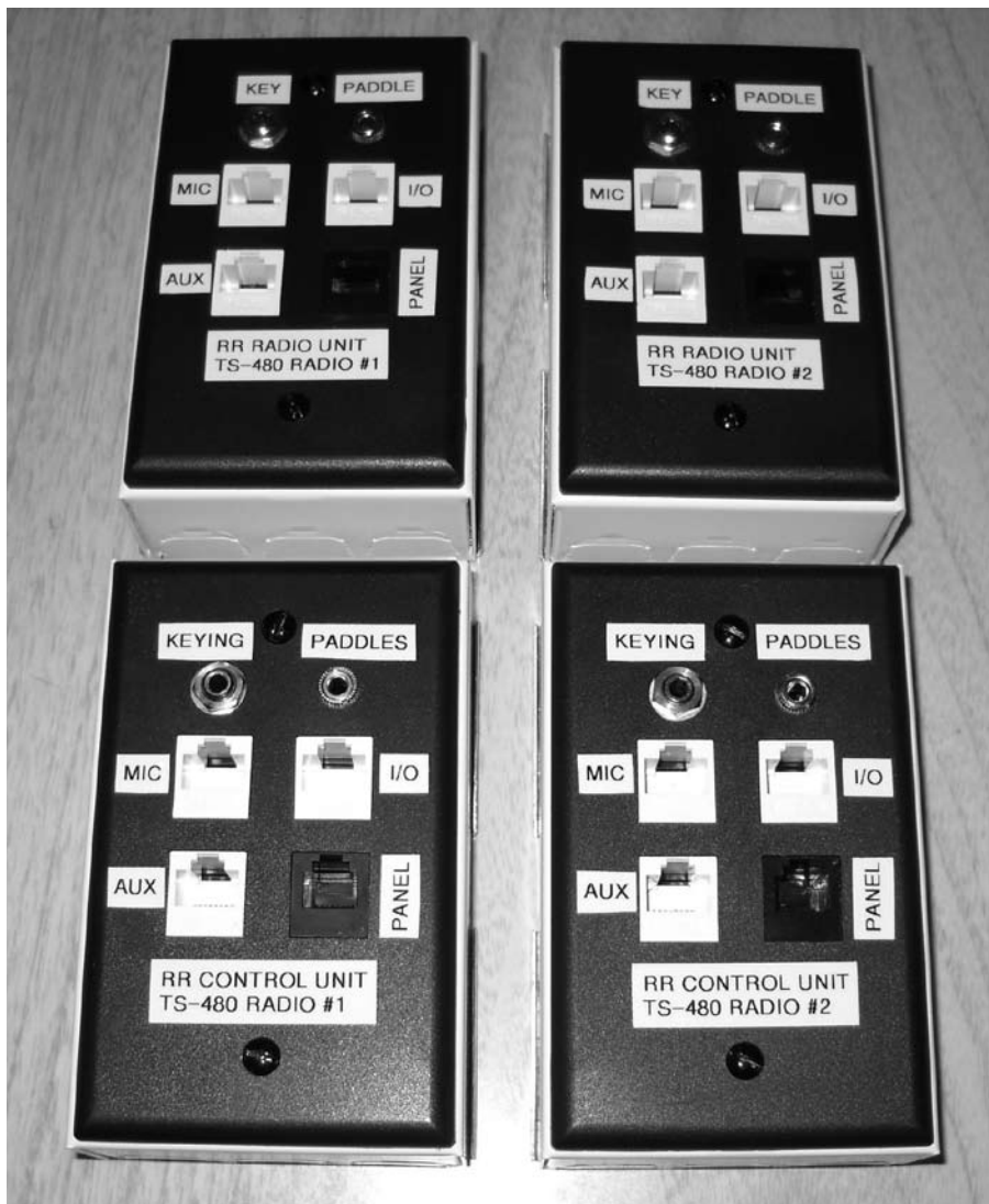
Figure 4 — Locust custom patch boxes for Remoterig connections
