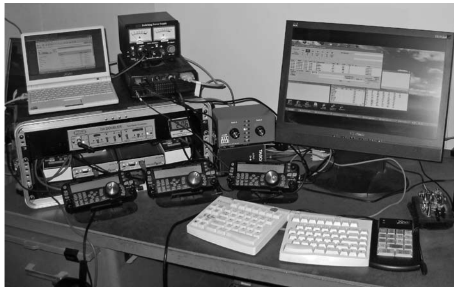
Figure 9 — SO2R remote control integrated with the control point SO1R rig
