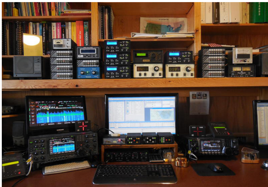
Figure 3 — The shack — perfect for SO2R and M2 operation. Either radio can grab any antenna instantly. A microHAM MK2R+ makes SO2R operation easy. I use DXBase for general logging and N1MM Logger for contesting. [Glenn Johnson, WØGJ, photo]
