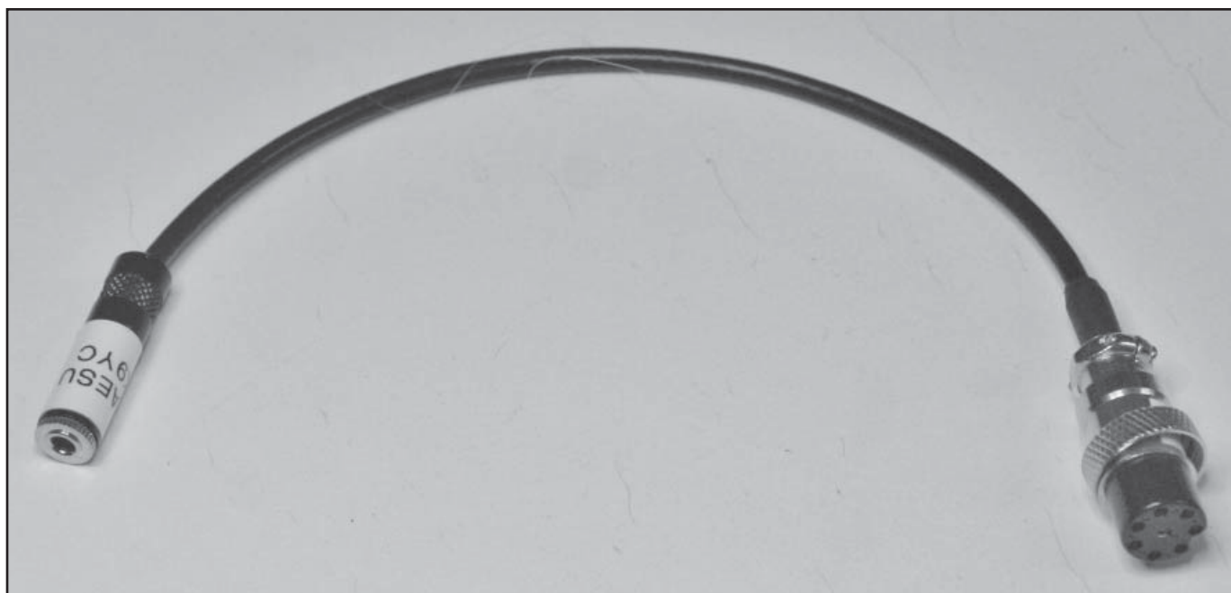
Figure 1 — Adapter to connect computer microphone to Yaesu (see text).
