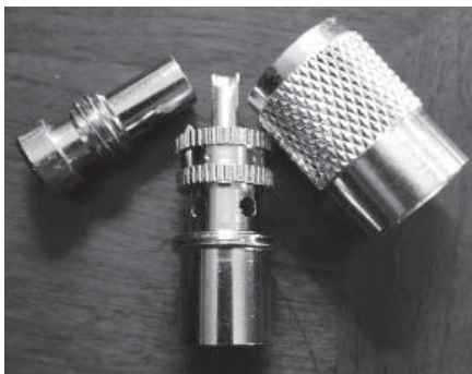
A typical PL-259 with a UG-175/U adapter for smaller-diameter coax. [Rick Lindquist, WW1ME, photo]
