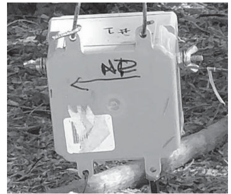
Figure 3 — Weather-proof box for outdoor use with a cover that is protected with gaskets
