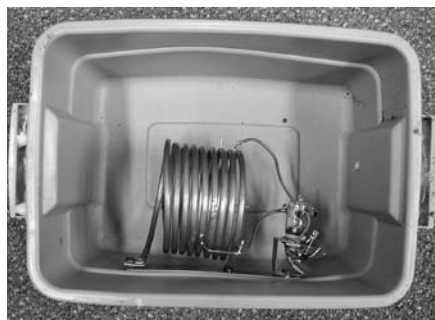
Figure 3 — Relay and base inductor example
