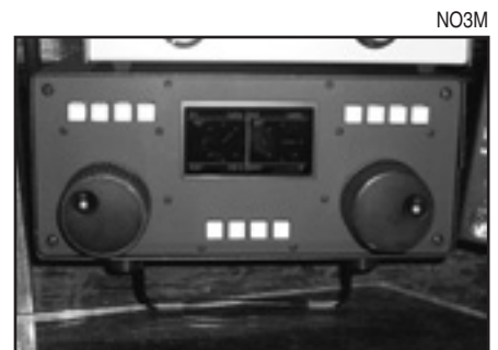
Figure 6 — The desktop controller sends serial data over an RS-485 network to slaved switch controllers.
