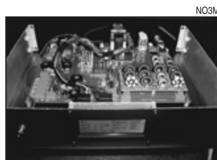
Figure 8 — The signal-processing unit with its top cover removed
