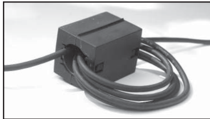
Figure 6 — A 5-turn choke, suitable for 7 MHz to 30 MHz.
