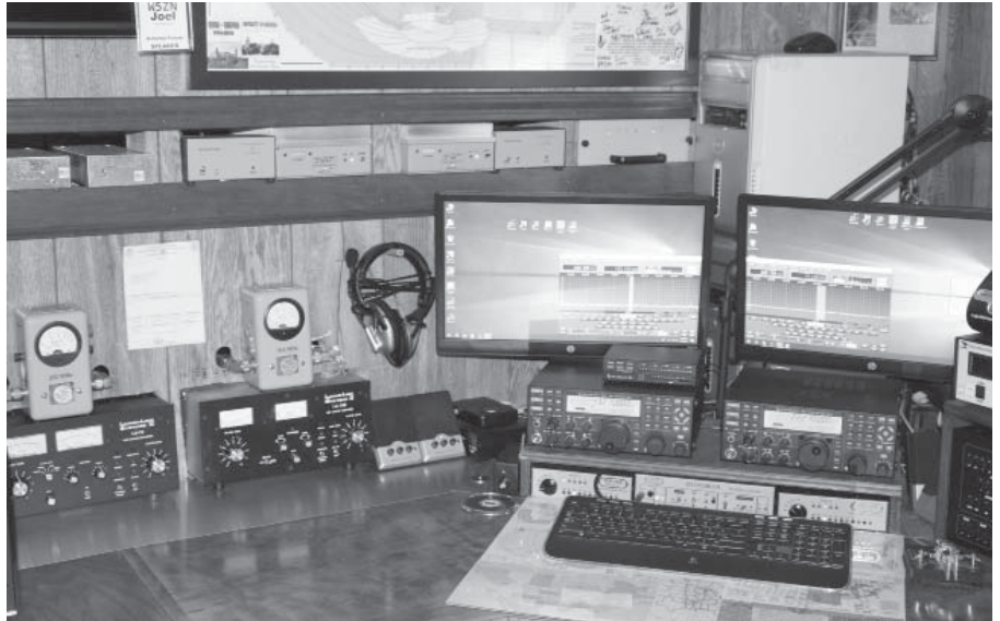
Figure 1 — The 222-MHz and 432-MHz station at W5ZN. Elecraft K3s serve as the IF radio for Downeast Microwave transverters (near the top of the photo) with Lunar Link amplifiers to the left of the K3s.
