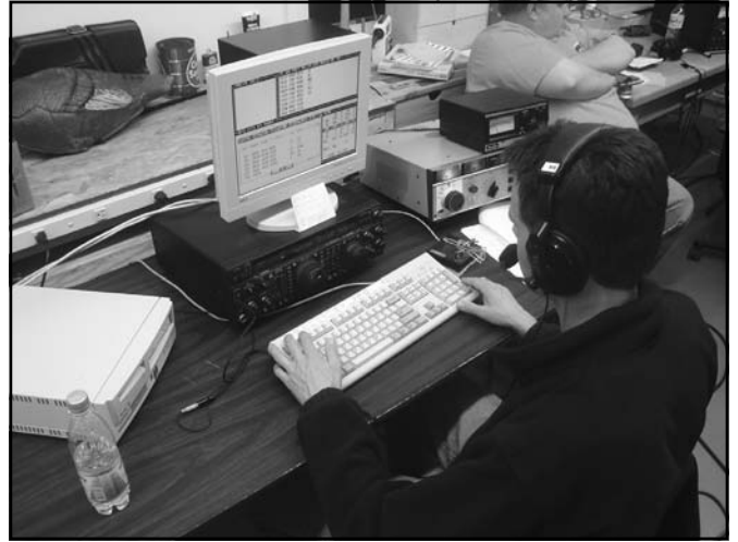
Fig 7—The 20 meter station with Uli, KK8I, at the controls. A FT-1000MP drove a Ten-Tec Titan amplifier, and the antenna was a 3-element Yagi.
