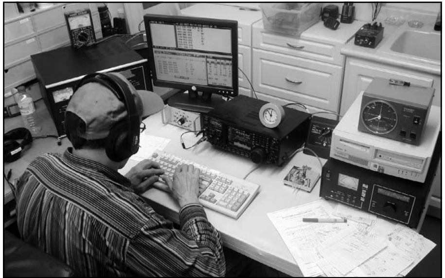
Fig 8—The 80/15/10 meter station with W8MJ at the computer keyboard: The rig was KN8S’s IC-756PROIII driving his AL-1200 amplifier through W8MJ’s IC-419 multiband bandpass filter. The Alpha-Delta coax switch, at the right of the transceiver, selected either the 15 or 10 meter Yagi or the 80 meter.
