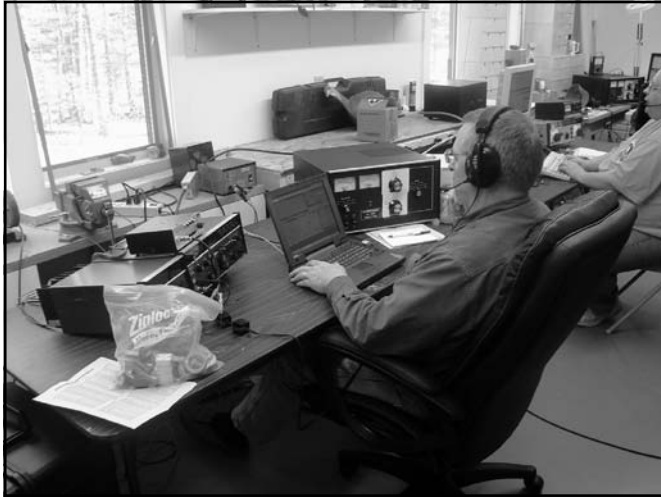
Fig 6—The 40 meter SSB station with KE8OC at the mic: The Corsair and its power supply are on the left, and W8MJ's AL-1200 amplifier is on the right. K8CC's MFJ-432 voice keyer sits atop the Corsair.
