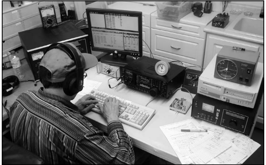
Fig 8—The 80/15/10 meter station with W8MJ at the computer keyboard: The rig was KN8S’s IC-756PROIII driving his AL-1200 amplifier through W8MJ’s IC-419 multiband bandpass filter. The Alpha-Delta coax switch, at the right of the transceiver, selected either the 15 or 10 meter Yagi or the 80 meter.
