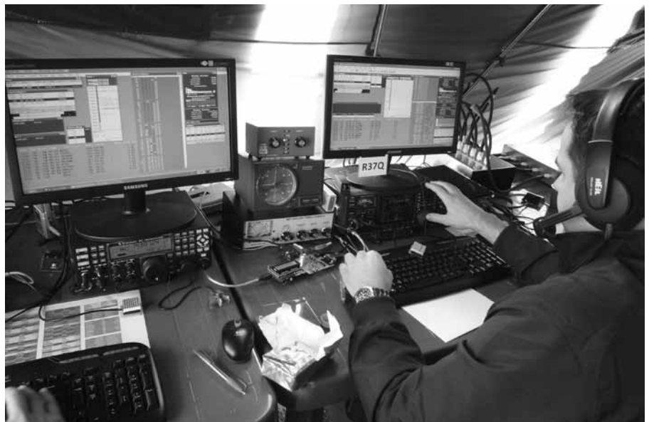
Figure 3 — A typical operating position: At R37Q, ops 5B4WN and 5B4AFM used a K3 and an IC-756, plus Win-Test for logging.
