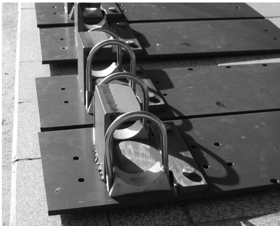
Figure 2 — Anodized aluminum boom cradles fabricated using DX Engineering parts and homebrew pieces by N8LGP for side-mounting Yagis have survived the severe climate
