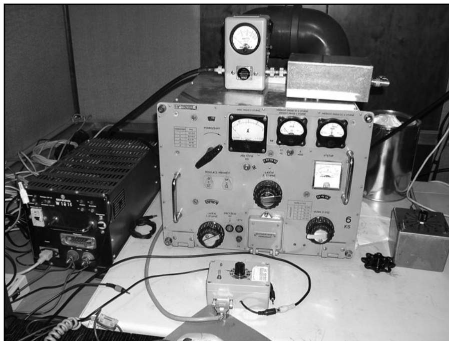
Figure 4 — The surplus Russian amplifier with "auto tuning"
