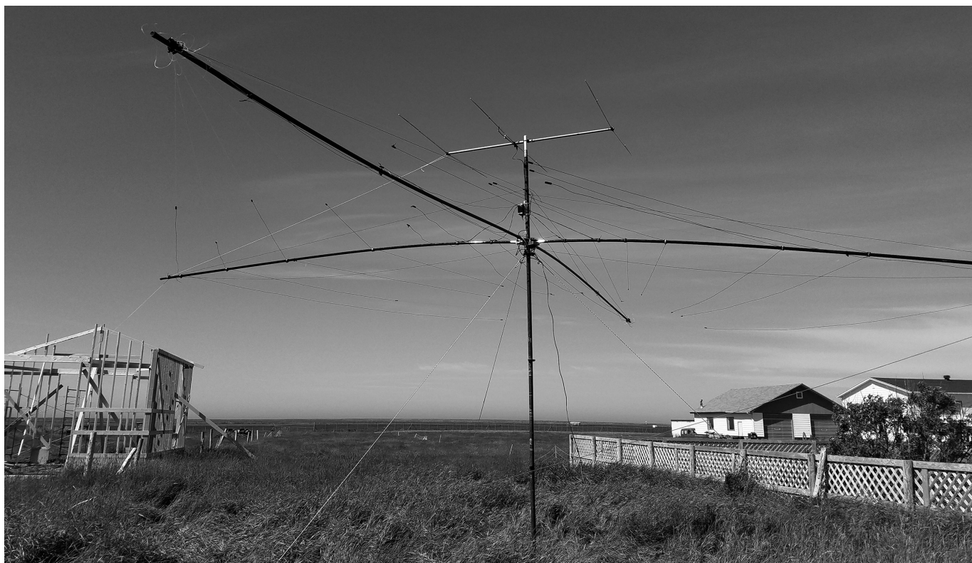
A low SpiderBeam survived the winds on Miquelon to keep Eric, FP/KV1J, on the air. [Eric Williams, KV1J, photo]
