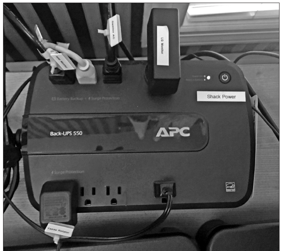
An example of a UPS.
