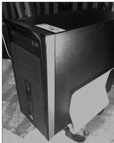
Placing a tower computer on a stand helps to avoid any floor issues and enhances air flow for cooling.
