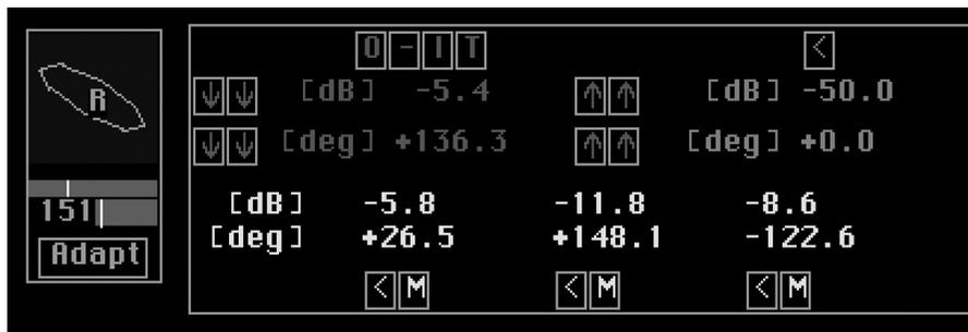
Figure 2 — The left side of the screen is the *Linrad* polarization graph, which displays phasing and amplitude balance. It's also used to set the time constant of the adaptive receive mode. The polarization window displays amplitude and phase difference between the two channels numerically. You can also stop the adaptive function and use the controls in this window to manually adjust amplitude and phase.
