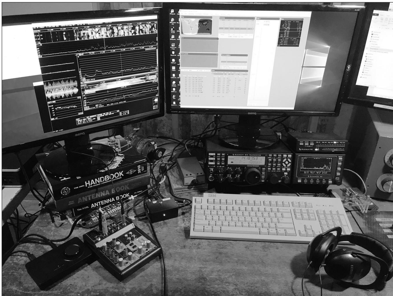
Figure 4 — My station running *Linrad* during the 2019 WPX SSB. The three boxes specific to using *Linrad* (left to right) are the Asus Xonar USB sound card, used as *Linrad* audio output; the Xenyx 502 mixer console, and the *Linrad*/K3 audio switchbox. Not shown is the very small Airspy HF+ SDR, plugged into the IF OUT port of the K3.
