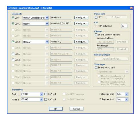
Note: Even though the SO2Rxlat has an LPT-looking port, do NOT check the LPT box
