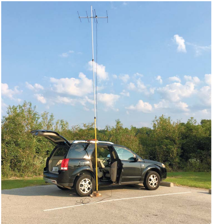
The initial K5ND rover set up using a painter pole and rooftop straps.
