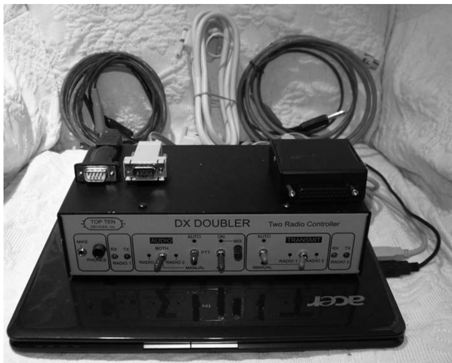
Figure 2 — Using the PIEXX SO2Rlat in conjunction with a serial-to-USB adapter, Win-Test was able to support the LPT-based DX Doubler. In addition, serial connections were available for CAT control of two radios.
