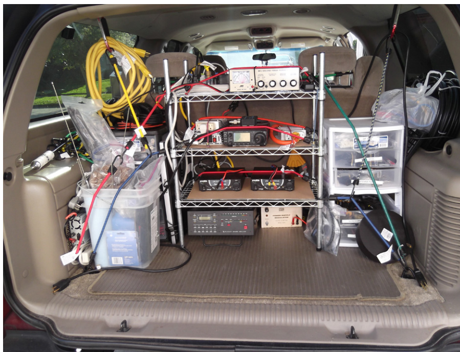
Figure 2 — The dc power rack, parts, and tools storage.
