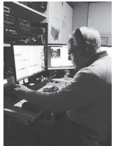
Figure 3 — Lee, KY7M, searches for a mult. Three computer screens were used: Left for N1MM+ , center for TeamViewer , and right for DXAtlas , to watch the grayline.
