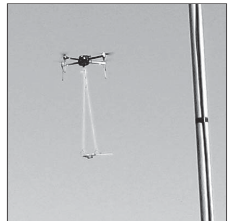
Figure 4 — IRIS+ quadcopter equipped with a receiving array to measure signal strength at various take-off angles.
