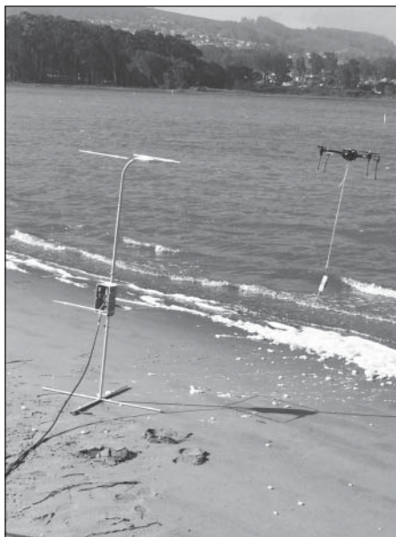
Figure 5 — Antenna set up for testing take-off angles over salt water.
