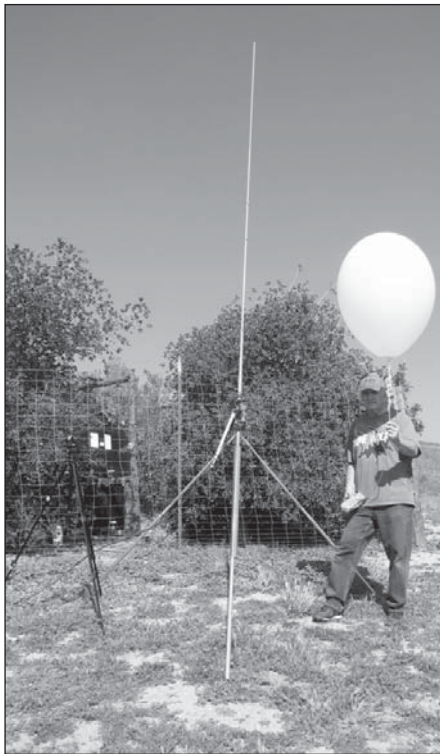
Figure 2 — The author with a helium-filled large-diameter balloon used for measuring take-off angle radiation patterns in vertical arrays.
