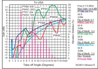
Figure 15—Responses for Top Four stations toward the USA on 40 meters. PT5M seems to have really exploited its advantageous terrain at low elevation angles toward the USA.
