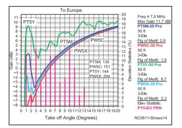
Figure 14—Responses for Top Four stations toward Europe on 40 meters. PT5Y doesn't appear to have made more QSOs because of a better terrain profile in that direction.
