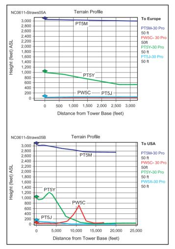
Figure 5—At A, a "true-perspective" view of the terrain profiles toward Europe from the Top Four WRTC 2006 stations, using equal scaling on both x- and y-axes. The PT5Y terrain slopes down such that the equivalent height of the tri-bander antenna on 15 meters was about 65 feet, compared to the actual physical height of 50 feet. At B, HFTA terrain profiles toward the USA.
