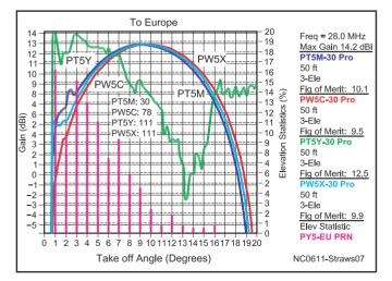
Figure 7—*HFTA* response for Top Four stations toward Europe on 10 meters. The table of numbers shows the QSOs into Europe for each station. PT5Y would appear to have an advantage by about 2.5 dB on average over all the statistically relevant elevation angles.
