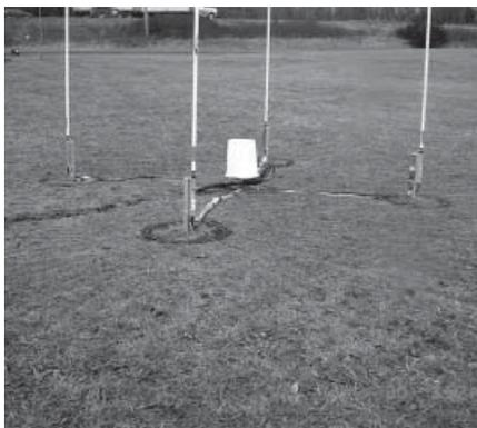
**Figure 2 — A short vertical receive array at K3LR. This array is actually for 10 meters (which fits well into a photo).**
